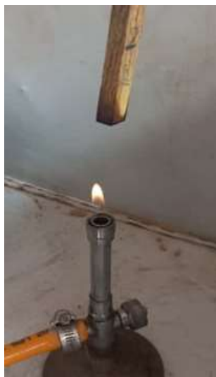
Fig. 2. Vertical burning testing set.
