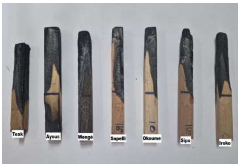
Fig. 6. Appearance of test samples after LOI test.
