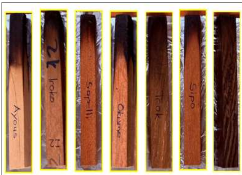
Fig. 4. Appearance of test samples after flammability test.
