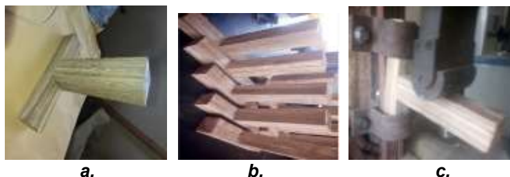
Fig. 6. Laminated bamboo joints samples a and b - Laminated bamboo joints samples; c - Joints samples held with fabricated jig during experimentation.
