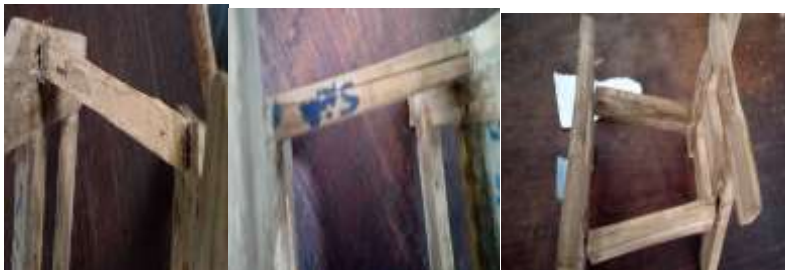
Fig. 16. Mode of failure observed in model frame after experimentation.
