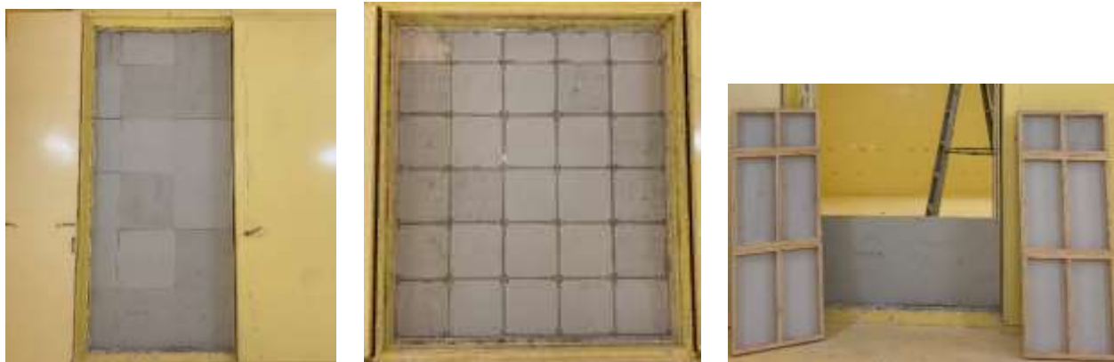
a. The specimen of composite wall of 5.1 m 2 .
