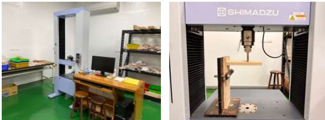
Fig. 3. Autograph AG-10T Universal Testing Machine.
