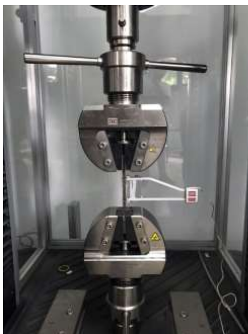
Fig. 13. Tensile testing of the composite material produced from bamboo-PLA-TPU materials under a certain load using an extensometer.
