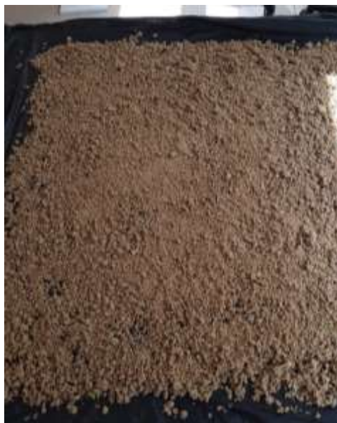
Fig. 7. Drying of bamboo fibers at room temperature.
