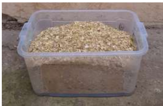
Fig. 3. Soaking coarse bamboo chips in water.
