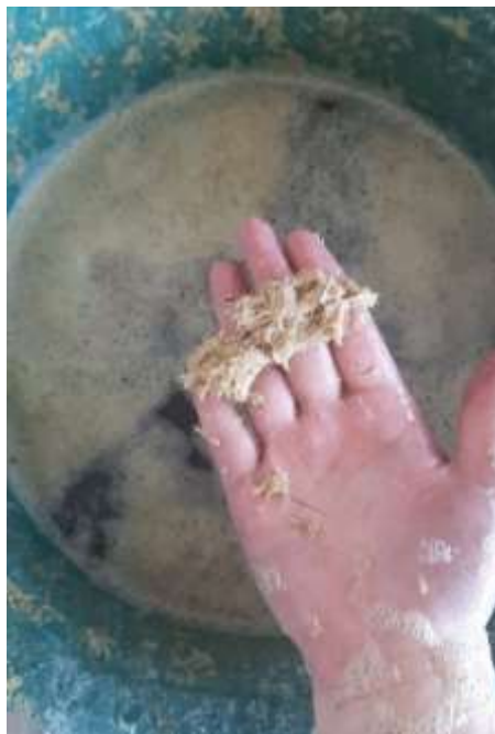
Fig. 5. Bamboo undergoing fibrilization process in refinery.
