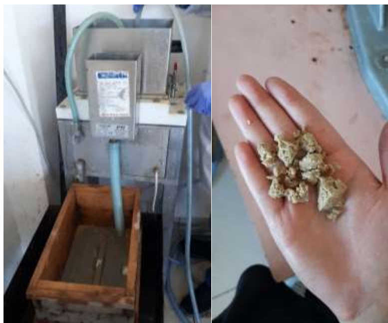
Fig. 6. The process of filtering the fibrillated bamboo fibers in the refiner.
