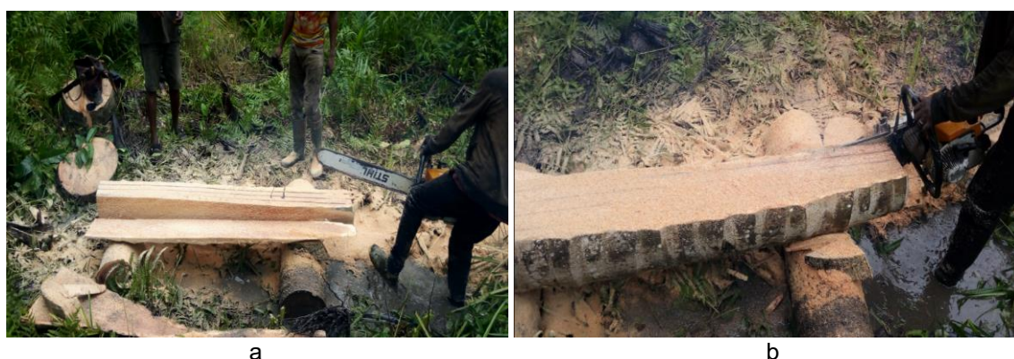
Fig. 2. Conversion of the coconut stem sections into planks. This stem was converted from the outer zone to the inner zone.
