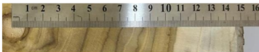
Fig. 6. Evaluation of heartwood and sapwood of teak.
