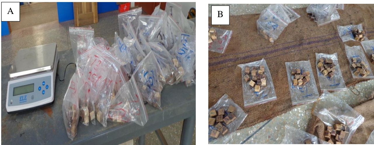
Fig. 1. Cubes packaged for weighing on scale (A), saturated samples removed from water for volume measurements (B).
