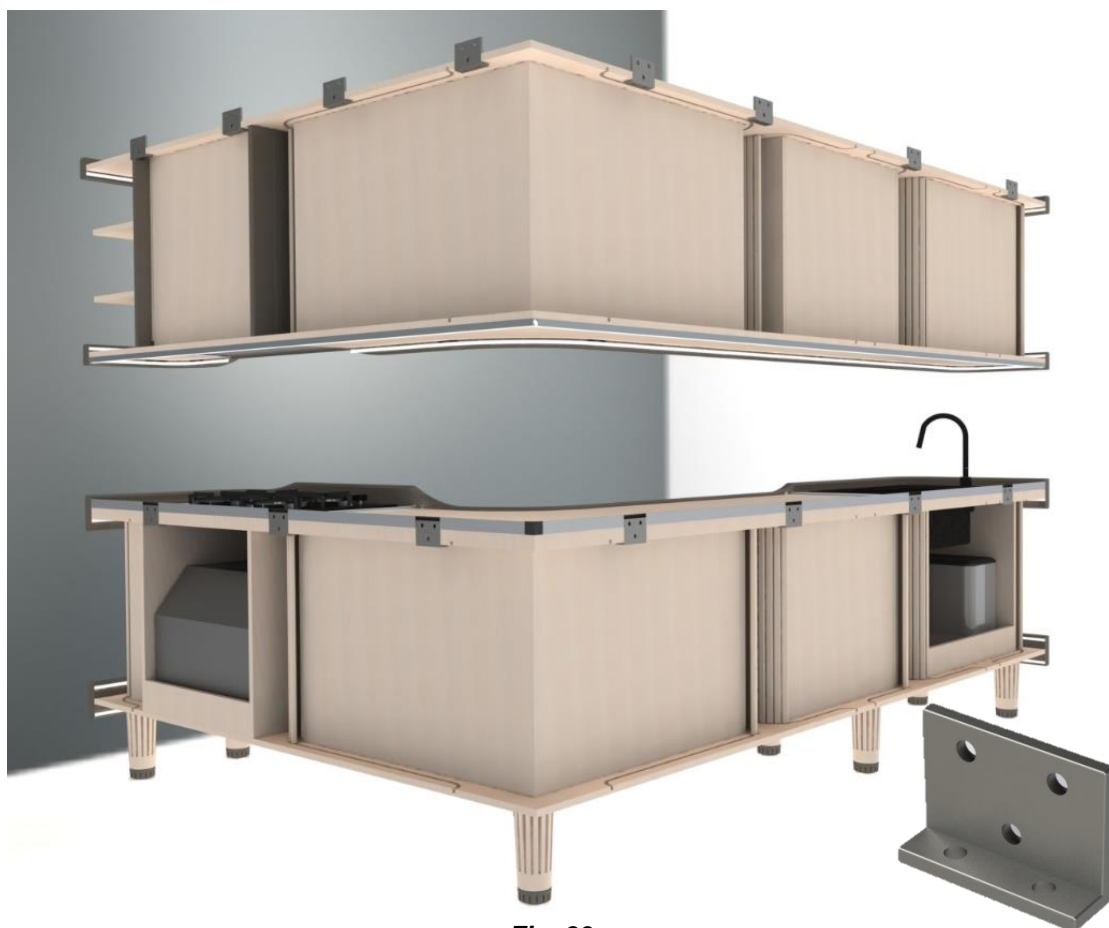
Fig. 39. Metal corner profiles for suspending the structure.
