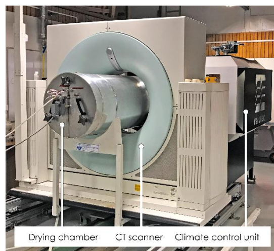
Fig. 2. X-Ray CT Scanner and Research Kiln Setup.
