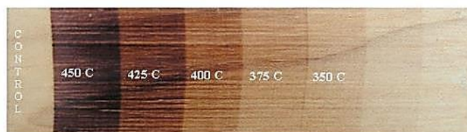
Fig. 2. Sample NL2, showing the effect of heating on wood colour.
