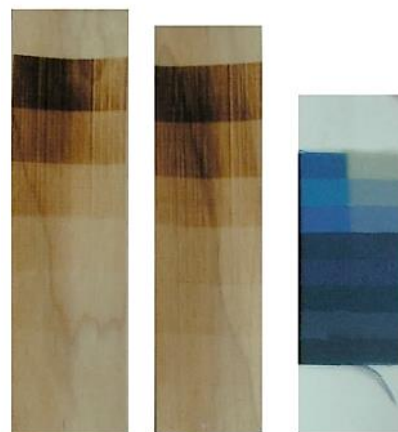
Fig.10. NL1 and NL2, after 110 days, with the blue wool fading card.
