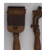
Fig. 10. Pore roller with feeder and unwinding roller.
