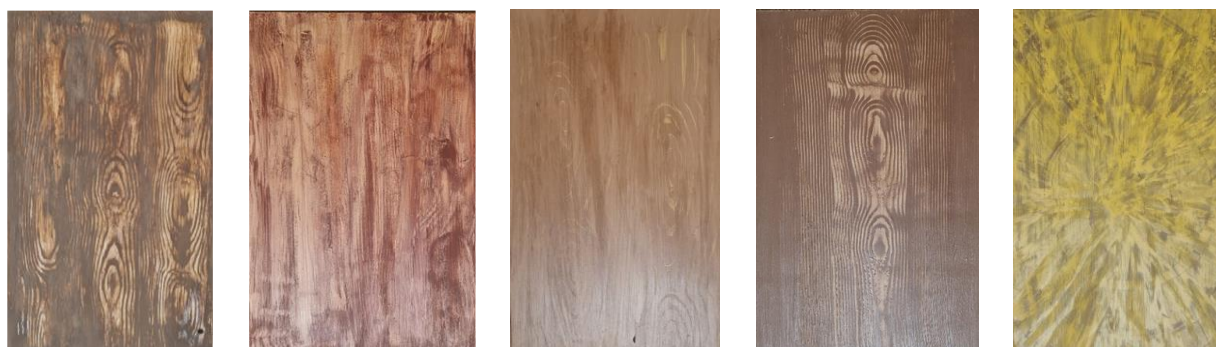
Fig. 26. Flader finishes made by stamps or free hand, imitating the tangential surface or annual rings.
