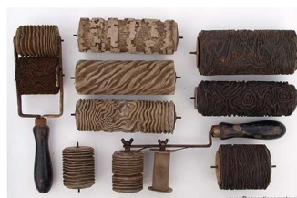
Fig. 12. Rollers types (a- old grain roll made of leather, b- rubber grain roller).
