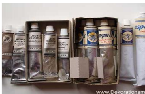
Fig. 4. Glaze paint for graining from Kaspar and Worrtsch ( www.dekorationsmalerei.at ).
