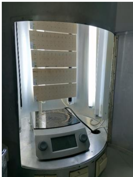
Fig. 3. Photocatalytic reactor used for aging process.
