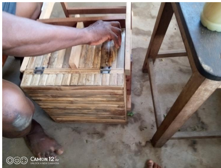
Fig. 2. Assembling of side aprons using Bamboo strips.
