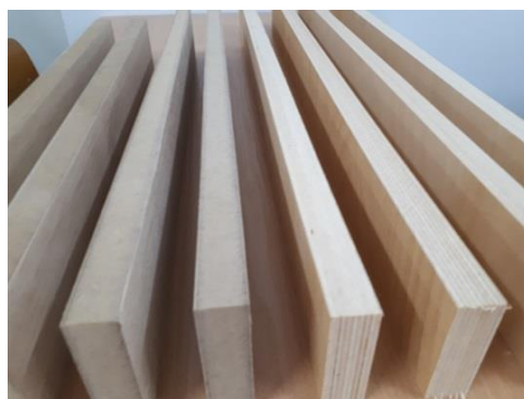
Fig. 3. Plywood and MDF test samples.
