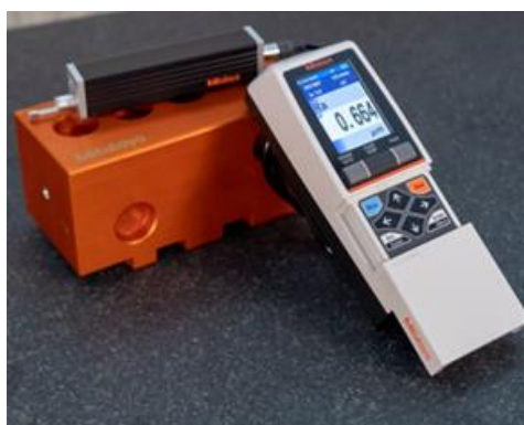
Fig. 4. General view of profilometer SJ-210, Mitutoyo, Japan ( https://mitutoyo.eu ).
