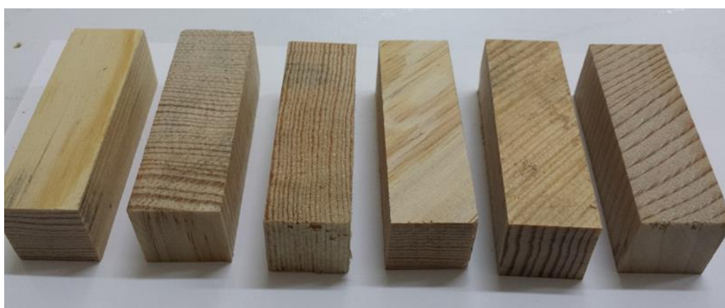
Fig. 2. Compression test samples (Control samples).
