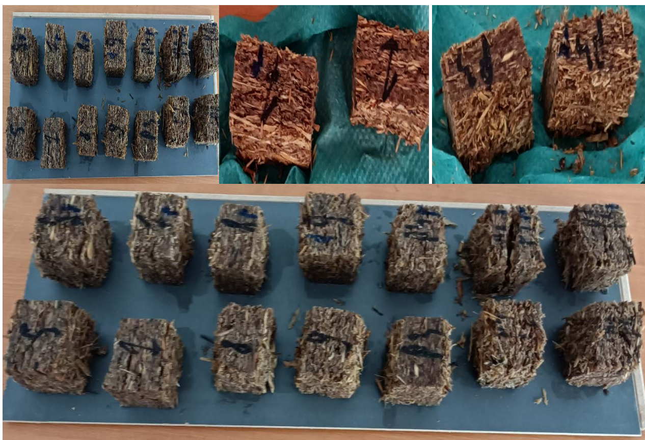
Fig. 5. Samples after 24 hours of water immersion.
