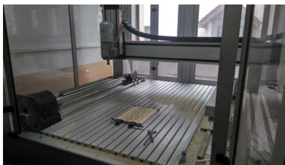
Fig. 4. CNC router used to process the panels.
