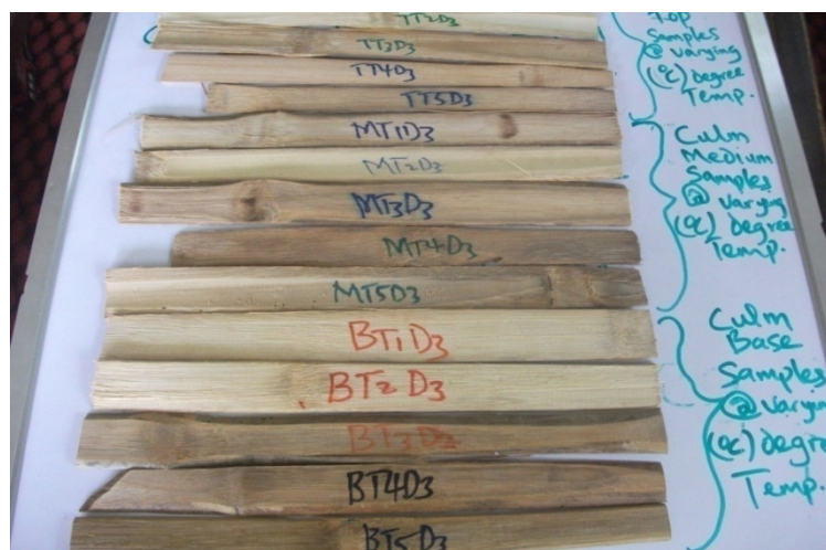
Fig. 1. Colour variations in the thermal treatment of Bambusa vulgaris .
