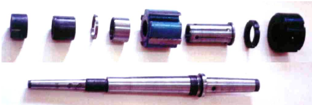
Fig. 3. Tool clamping system with conical mandrel for the MNF10 milling machine.
