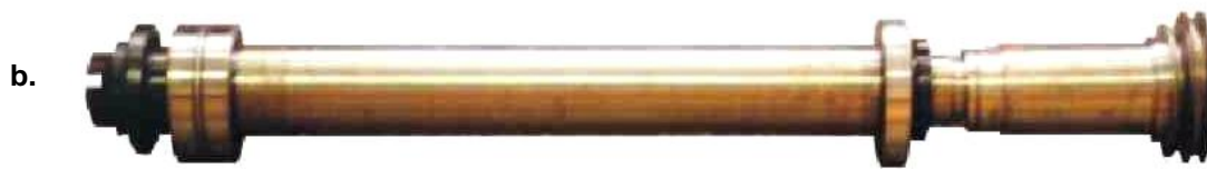
Fig. 2. The working shaft of the MNF10 milling machine: a. the classic variant, before the modification; b. the improved variant, after the modification.
