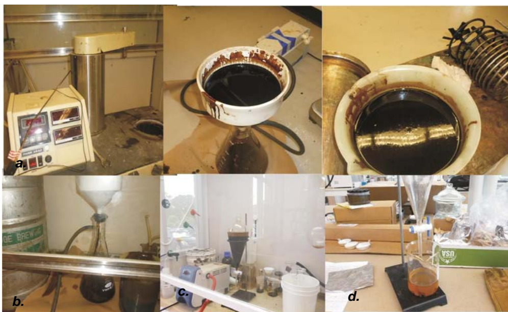
Fig. 2. Liquefaction reactor (a) used to separate the liquefied fraction under vacuum (b) and subsequent separation with the use of separatory funnel (c) to obtaining the bio-oil (d).
