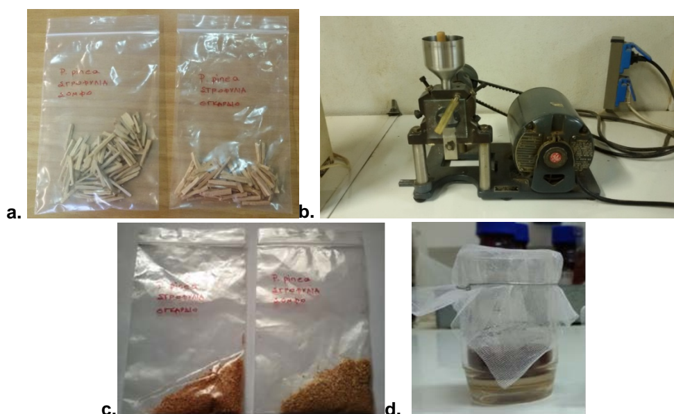
Fig. 3. The stages of the extraction of the samples; starting material after trimming with Wiley's mill: a. wood after cut in sticks with knife; b. Wileys' Mill used for trimming; c. wood dust after the use of Wileys' Mill; d. wood dust in glass ready for Soxhlet device.
