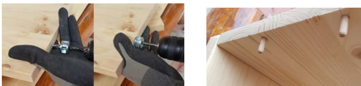
Fig. 6. Drilling the lateral walls and the inferior plate.
