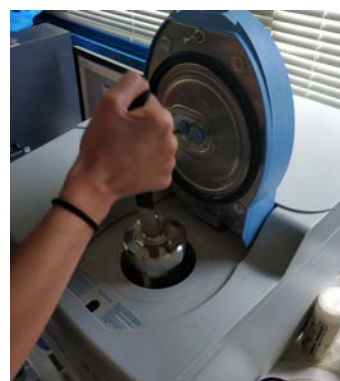
Fig. 6. Final step, inserting the bomb into the apparatus.
