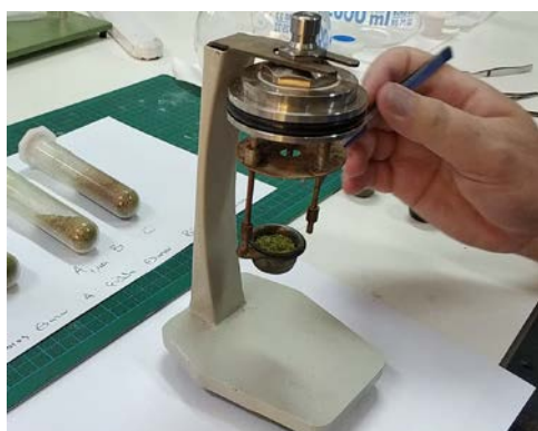
Fig. 4. Having compacted the powdered sample into the capsule and attached the ignition thread.
