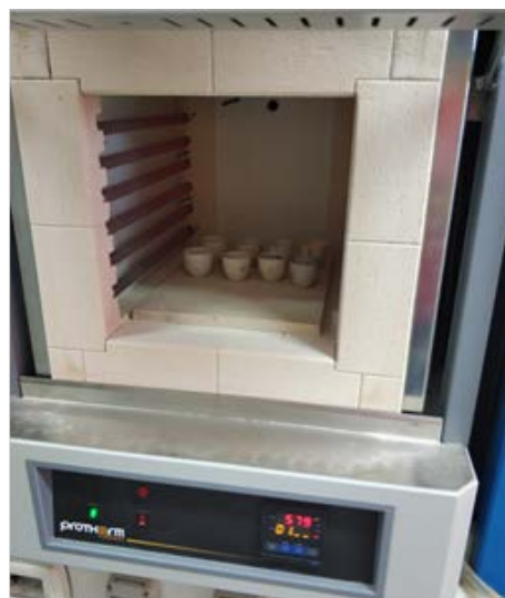
Fig. 5. The samples positioned into the furnace.
