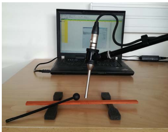
Fig. 2. Microphone AUDIX TM1PLUS used to capture the beating of samples, rubber mallet and a Padouk specimen.
