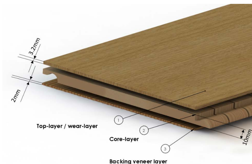
Fig. 1. Structure and dimensions of multi-layered parquet elements produced in this study.
