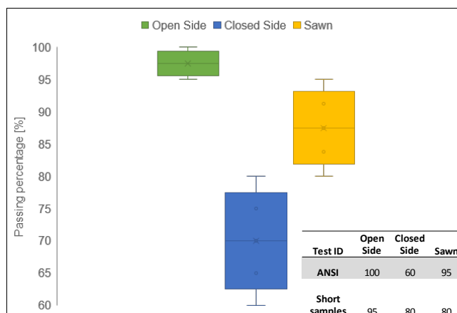
Fig.8. Rate of specimens passing the delamination test depending on the top-layer material; the table represents raw test results.
