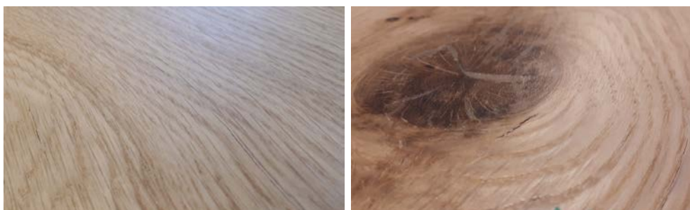
Fig. 5. Slicing checks on the surface of clear wood (left) and around knots (right).
