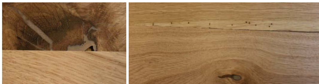
Fig. 4. Example of edge tear out due to edge-filled knots (left) and sapwood (right).
