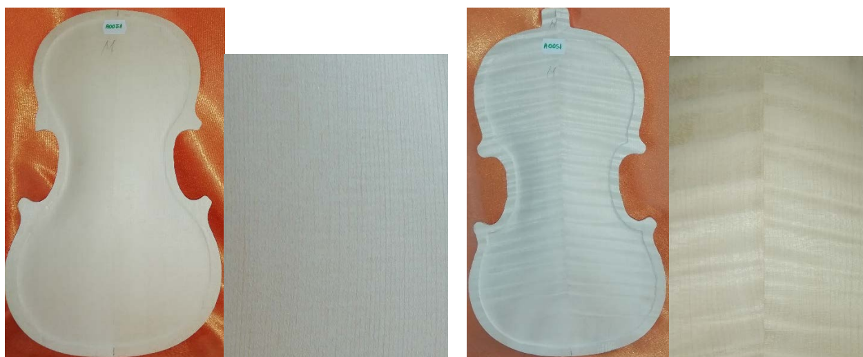
Fig. 2. Violin plates – top plate (a) and back plate (b).
