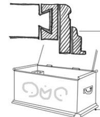
detail of a wooden chest tongue and groove joints
