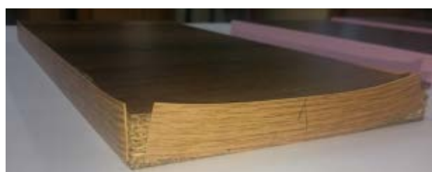
Fig. 4. Self-delamination of PVC edge from edge banding compound after impact of high temperature.
