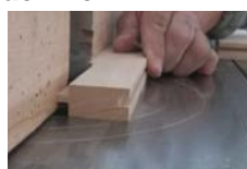
h). groove milling – normal/vertical axis milling machine (MNF); 5mm mill
