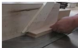
g). groove milling – normal/vertical axis milling machine (MNF); 5mm mill
