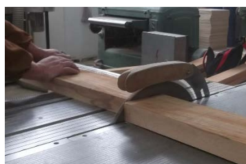
a) severing – circular saw
