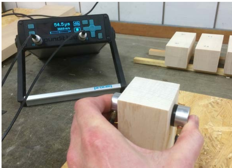
Fig. 4. Ultrasound measuring device Proceq Pundit Lab.
