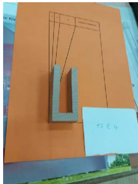
EDS-treated wood without red heart: 0.8 / 0.5 (average = 0.65)
