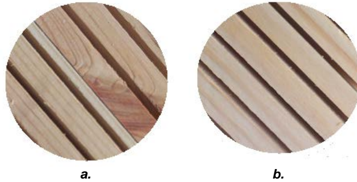
Fig. 3. Structural difference of specimen surface in material parallel direction: a – with air gap between lamellas; b – without air gap.
