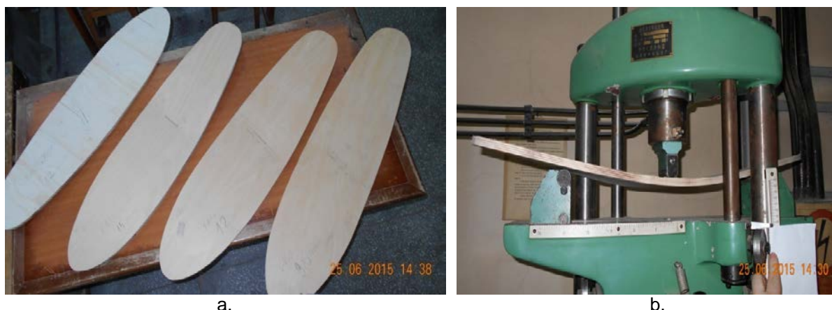
Fig 3. Longboard samples (a) and the determination of deformation (b).
