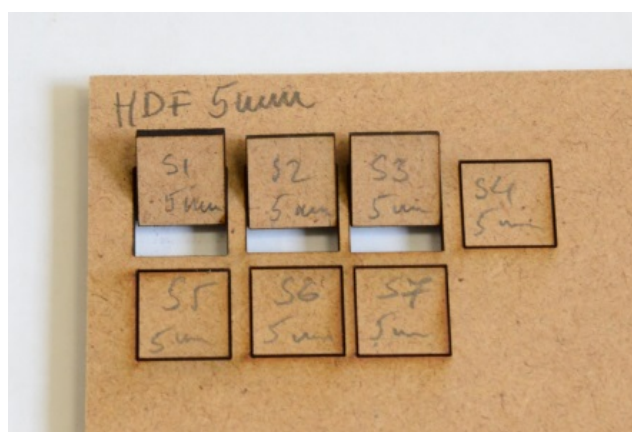
Fig. 5. 5mm thick HDF not cut through at a speed rate of S4 (20mm/s).
