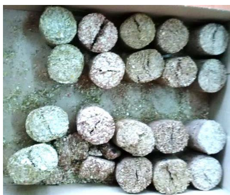
Fig. 7. Briquettes made from biomass, which were disintegrated after completing the compression testing.
