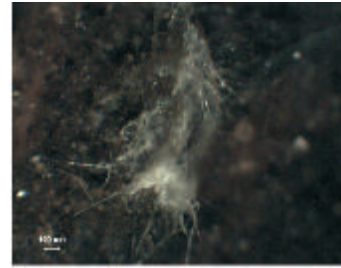
Fag netratat – mucegai alb 40x / Untreated beech - white mould 40x
